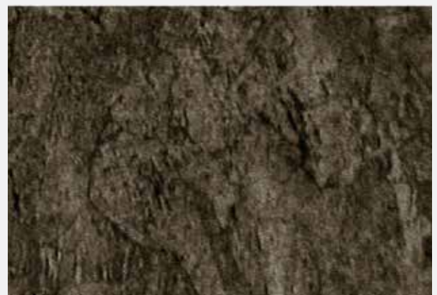
Luvata's CuCrZr fine grain structure
