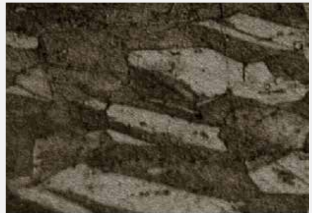
Conventional CuCrZr grain structure
