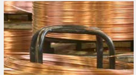
**Plating:** Luvata typically provides battery nail wire to the market 'pre-plated'. Plating is typically in the range of 0.5-2.0 microns of Bright Tin. Bare wire (to be post plated by the customer after nail forming) is also available.
