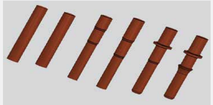
Connector cold-forming process
